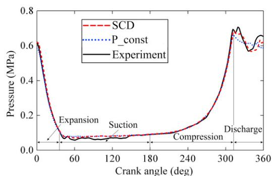
Fig. 2. In-cylinder pressure comparison between numerical and experimental data.
