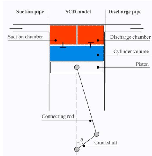
Fig. 1. Schematic of reciprocating compressor.
