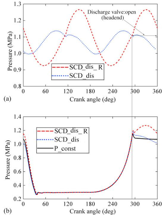
Fig. 4. Interaction between compressor and discharge system with or without resonance: (a) discharge pressure; (b) in-cylinder pressure.
