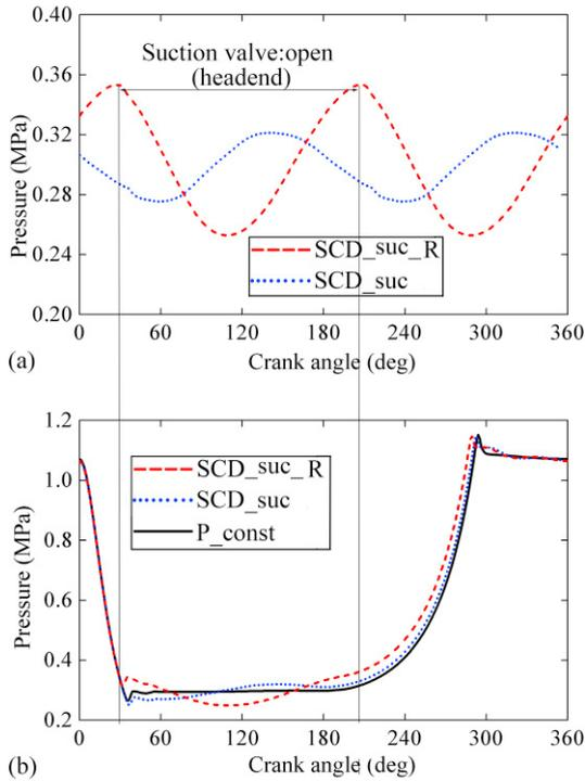
Fig. 3. Interaction between compressor and suction system with or without resonance: (a) suction pressure; (b) in-cylinder pressure.
